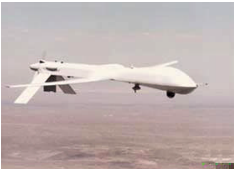
The Predator is 27 feet long with a wingspan of approximately 49 feet
